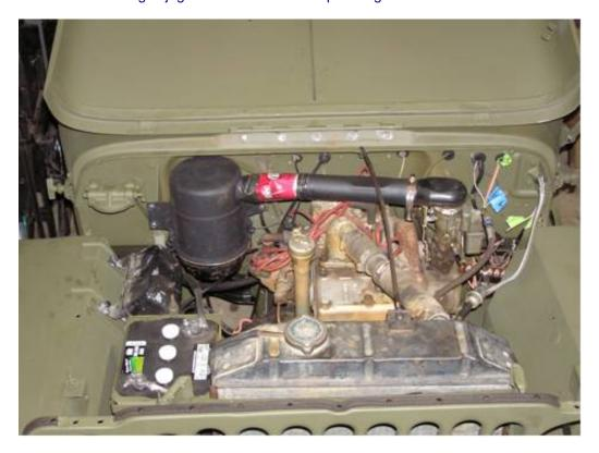
The "red" piece of the cross-over tube is a 20 oz. Dr. Pepper bottle ... taped and wired in place ... could not wait on the mail order part ...;-) (remember this "mod" for when something breaks in the field and you need an expedient hose of the like. No extra charge for the bail out.) The engine is running and I did not work on it.
