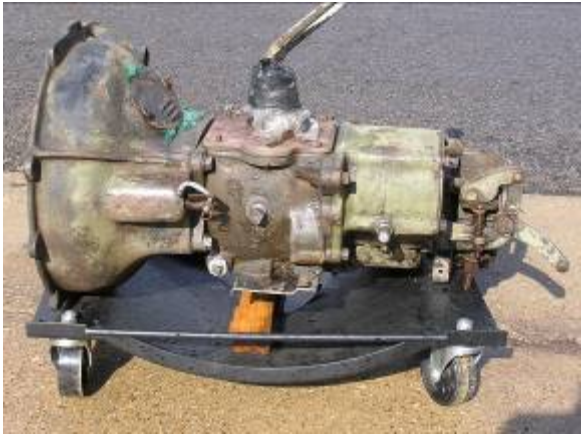
Transmission – After the first round of cleaning.
