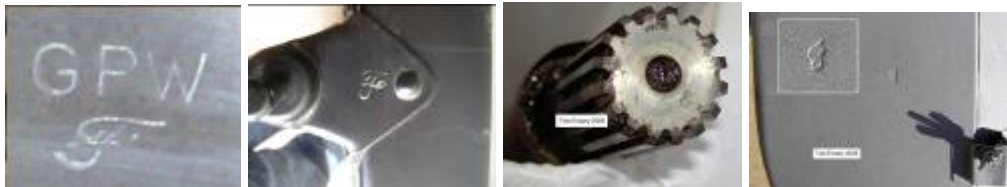
R-L Back side of engine/bell housing plate; Shock mount; End of propeller shaft; Right fender (one on the left fender also).
