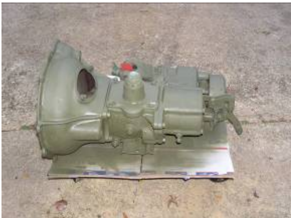
Transmission after cleaning and painting.
