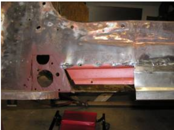
New body panel on the right ... new hat channel and ready to weld in the front body panel. Almost ready for the axe and shovel. The parts were primed when they were reached ... hoping that the rust would be abated for another 65 years!
